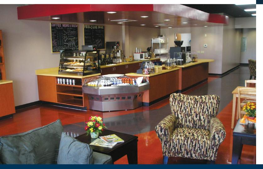
Metallix Floor™ incorporates a mixture of proprietary metallic aggregates and fluid applied resins to build a monolithic, durable, and chemical resistant seamless floor.
